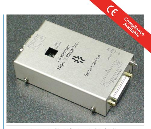
This microcontroller interface is offered as an option for Glassman High Voltage power supplies. Its purpose is to provide remote control capability of analog program signals, analog monitor signals, and digital control signals and monitors using standard RS-232 or USB interface computer control.
