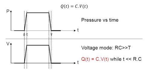
High impedance acquisition devices can be used. Total capacitor has to be considered (source capacitor, cable capacitor, device capacitor and optional additional capacitance).
