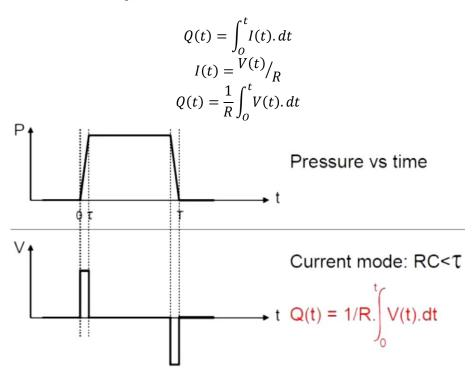
Numerical integration of this signal will give electrical charges delivered by the sensors. Digital data acquisition devices with high sampling rates are particularly adapted to the signal processing. If possible, it is recommended to measure the signal on two channels with different sensitivities.
