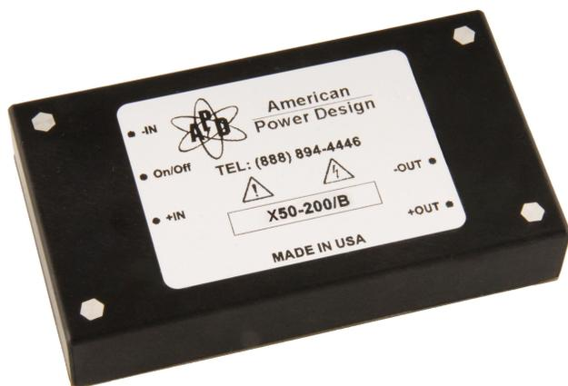
The X50 Series of DC/DC converters accepts ultra wide input ranges of 9-36 Vdc, 20-60 Vdc and 36-72 Vdc. Outputs are independently isolated. In the case of duals, up to 40 watts may be taken from either output. All models will tolerate a short circuit indefinitely. Also included is a Pi input filter and remote on/off.
