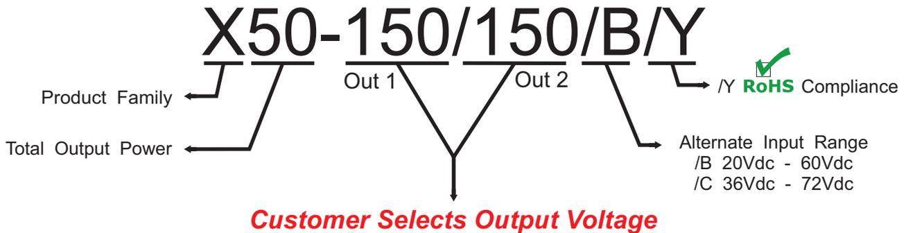
The X50 Series are designed such that the customer may order any output voltage from 48Vdc to 500Vdc at no additional charge.
