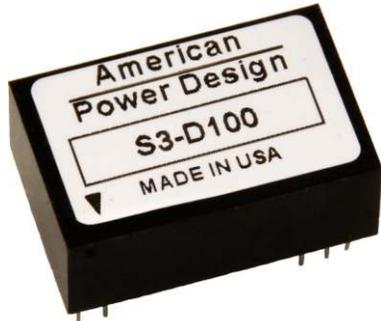
The S3 Series of DC/DC converters accepts an ultra wide input range of 9-36 Vdc, delivering a 500 Vdc isolated high voltage output. All models feature a 24-pin dip compatible configuration, continuous short circuit protection, and a low ESR input capacitor.
