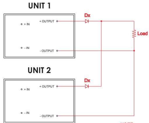
NOTE: The ratings of Dx should be 1.5 times the maximum current and voltage expected in each branch.
