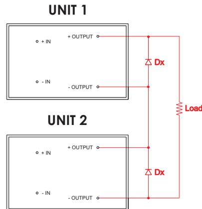
NOTE: The ratings of Dx should be 1.5 times the maximum current and voltage expected in each branch.
