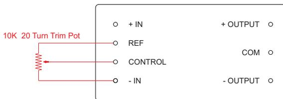
The figure below shows how to combine both of the prior configurations to form upper and lower boundaries for the adjustable range.
