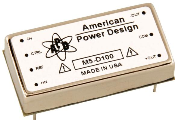
The M5 Series high voltage DC/DC converter offers 100% programmable single or dual high voltage outputs using a 0-5Vdc analog signal. Each model is enclosed in a six-sided shielded metal case and has 1000Vdc of isolation allowing one model to be utilized for both positive or negative applications. All models will tolerate a short circuit indefinitely.
