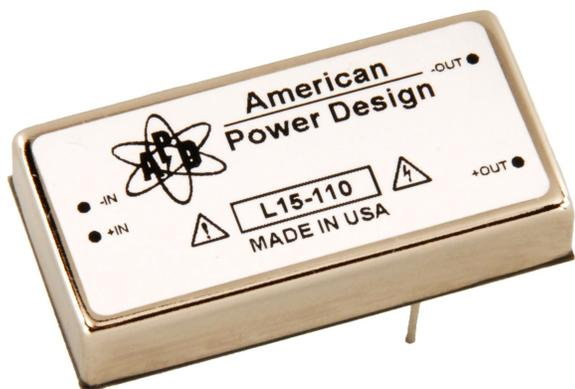
The L1 Series Low Profile DC/DC converter offers a 1000 Vdc isolated high voltage output in a six-sided metal case. Their small size, low output ripple, and excellent regulation characteristics make them ideally suited for applications that demand a high degree of performance. All models will tolerate a short circuit indefinitely.
