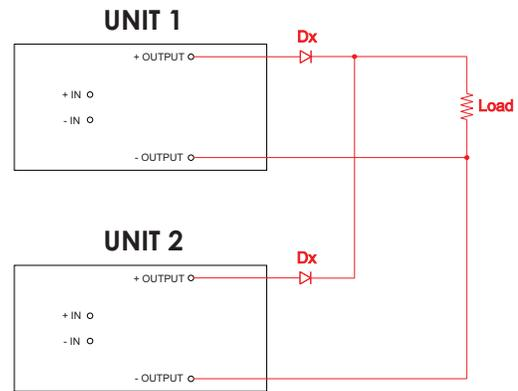
NOTE: The ratings of Dx should be 1.5 times the maximum current and voltage expected in each branch.
