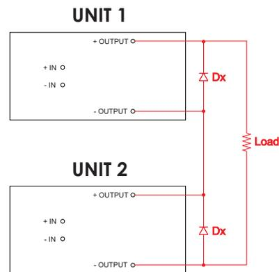
NOTE: The ratings of Dx should be 1.5 times the maximum current and voltage expected in each branch.
