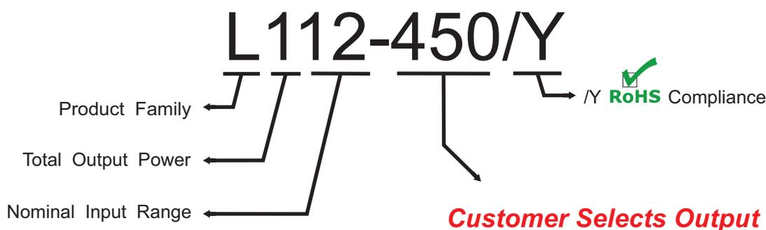
The L1 Series are designed such that the customer may order any output voltage from 24Vdc to 500Vdc at no additional charge.
