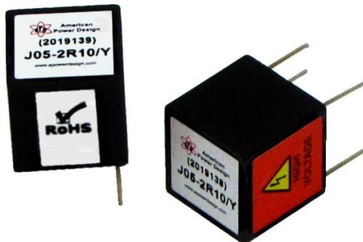
The J05 Series of miniature DC/DC converters offers a 500 Vdc isolated high voltage output directly proportional to input voltage. They are available in industry standard pinouts and a optional shielded case. These miniature converters are ideal for applications requiring minimal size and weight. All models will tolerate a short circuit indefinitely.
