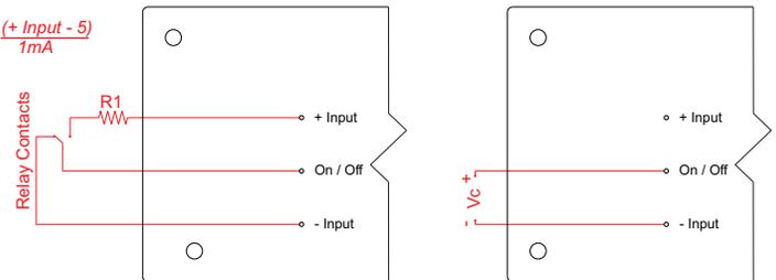
Converter Off:  $V_c > 3V_{dc}$
