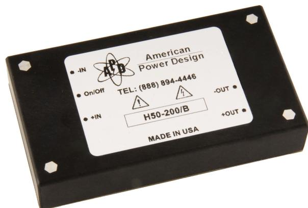
The H50 Series of DC/DC converters accepts ultra wide input ranges of 9-36 Vdc, and 20-60 Vdc. Outputs are independently isolated. In the case of duals, up to 40 watts may be taken from either output. All models will tolerate a short circuit indefinitely. Also included is a Pi input filter and remote on/off.
