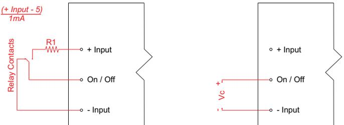
Converter Off:  $V_c > 3V_{dc}$
