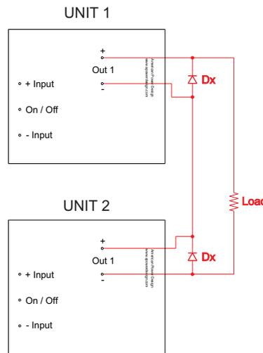
NOTE: The ratings of Dx should be 1.5 times the maximum current and voltage expected in each branch.
