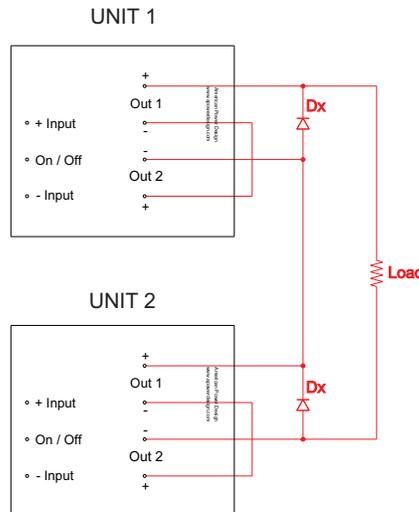
NOTE: The ratings of Dx should be 1.5 times the maximum current and voltage (Out 1 + Out 2) in each branch.
