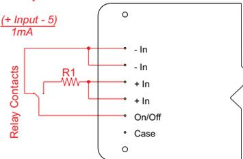
Converter Off:  $V_c > 3V_{dc}$
