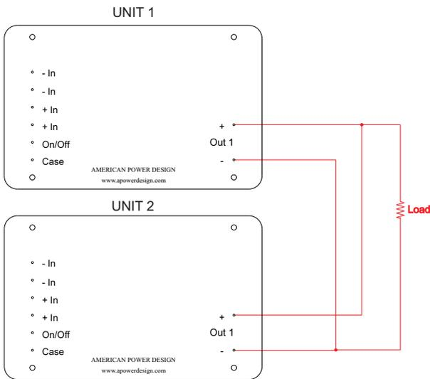
The figure below shows how to connect several dual output units with equal nominal output voltage in parallel.
