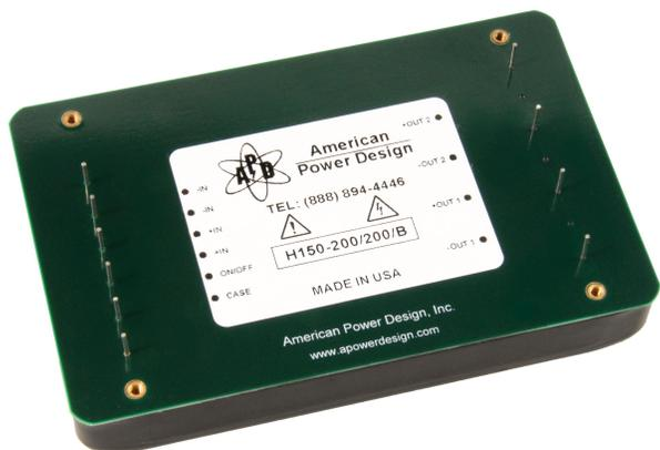
The H150 Series of DC/DC converters accepts ultra wide input ranges of 18-36 Vdc, and 20-60 Vdc. Outputs are independently isolated. In the case of duals, up to 120 watts may be taken from either output. All models will tolerate a short circuit indefinitely. Also included is a Pi input filter and remote on/off.
