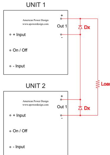
NOTE: The ratings of Dx should be 1.5 times the maximum current and voltage expected in each branch.
