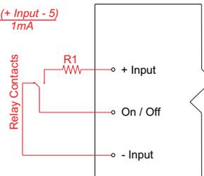
Converter Off:  $V_c > 3V_{dc}$
