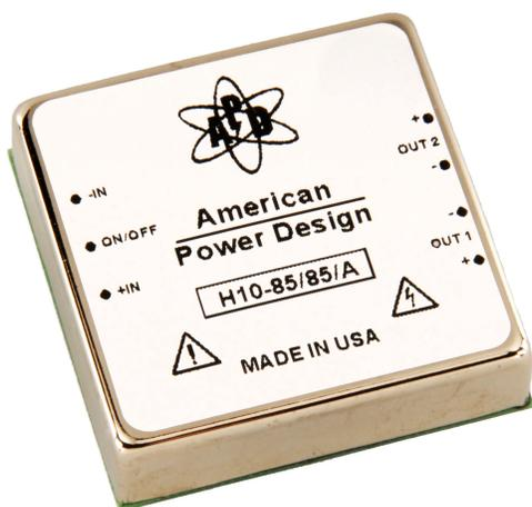
The H10 Series of DC/DC converters accepts ultra wide input ranges of 5-15 Vdc, 9-36 Vdc, & 20-60 Vdc. Outputs are independently isolated. In the case of duals, up to 4 Watts may be taken from either output. All models will tolerate a short circuit indefinitely. Also included is a Pi input filter and remote on/off.
