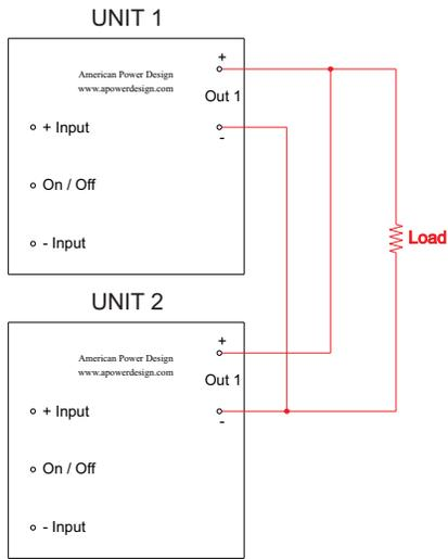
The figure below show how to connect several dual output units with equal nominal output voltage in parallel.
