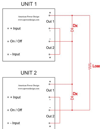
NOTE: The ratings of Dx should be 1.5 times the maximum current and voltage (Out 1 + Out 2) in each branch.
