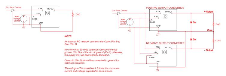
The figures below show standard configurations for the E1 Series converter with output voltages from 2.1kV to 4kV.
